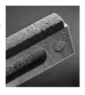
4. Low performance honing oil can create catastrophic welding between the workpiece and the mandrel shoe when honing soft materials ranging from stainless steel to low carbon steels. This may lead to serious and very costly problems such as: ruined honing tools, machine failure, part rejects and lost profits.
