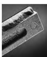
Honing oil with low lubricity or improper chemistry allows metal chips to lodge in the abrasive surface, much like mud in a snow tire. This embedded metal holds the abrasive surface away from the workpiece and slows down the cutting rate. Slower cutting rates decrease machine and operator productivity.
